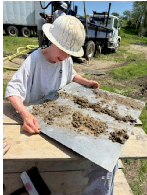
UNL-CSD Hydrogeologist, Susan Olafsen Lackey evaluating geologic samples collected from drilling a test hole in the Dakota formation near Martinsburg, NE.
